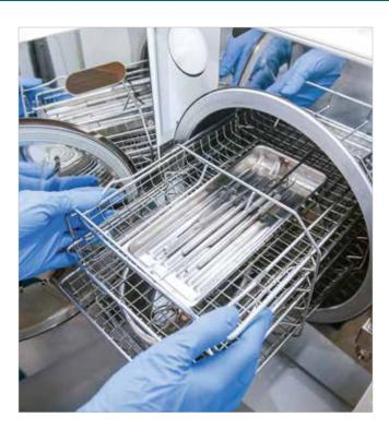
Autoclaves use steam and are either "gravity displacement" or "pre-vacuum" type sterilizers. Temperatures reach approximately 250° F to 273° F. Sterilization times range from four to 30 minutes depending on temperature, whether instruments are wrapped or unwrapped and the manufacturer's instructions for use. The "drying cycle" may be 25 to 40 minutes.
